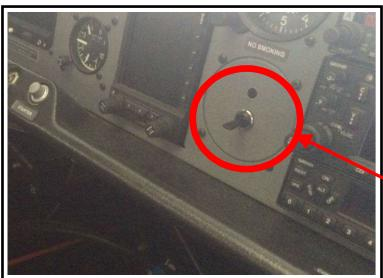
Flip the switch in OFF position
