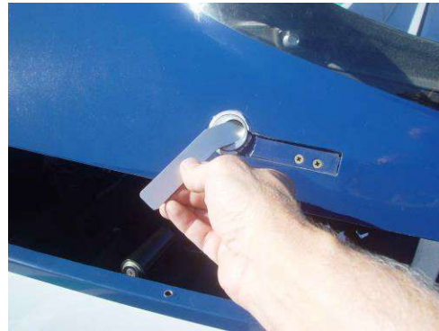
Rotate handle counter-clockwise to unlatch.
