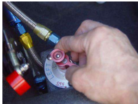
Lift center knob and turn lever 180 degrees.
