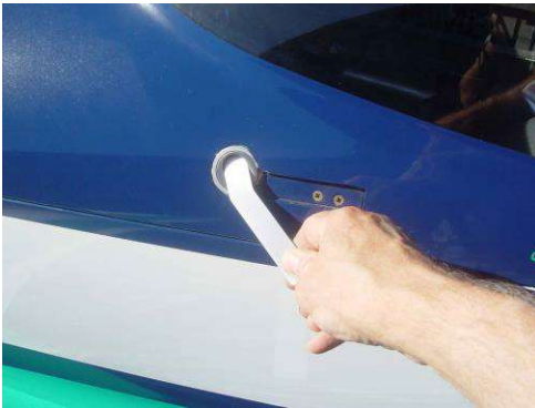
Rotate handle counter-clockwise to unlatch.
