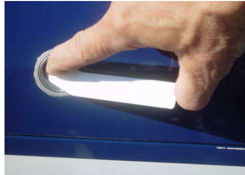
Press forward end and lift aft end of handle.
