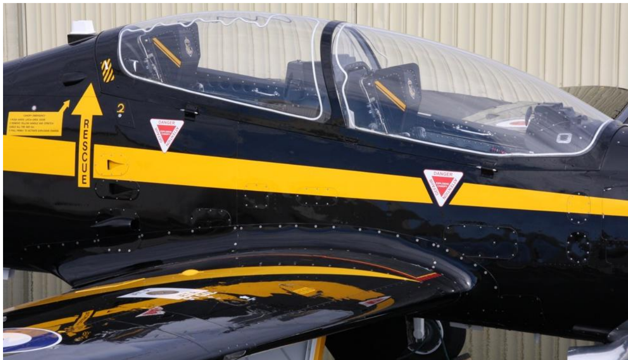
Figure 4: Yellow Stripped External Canopy Fracture Access Panel on the Canopy Rear (right side)
