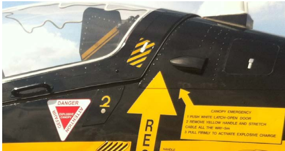
Figure 3: Yellow Stripped External Canopy Fracture Access Panel on the Canopy Rear (left side)
