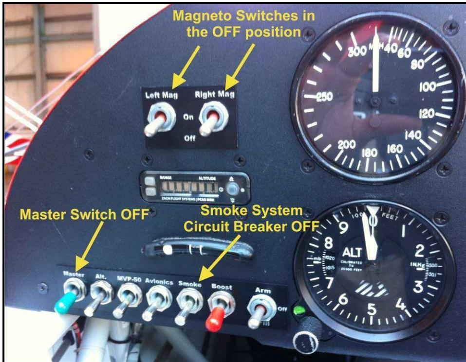
Figure 5 - MAGNETO switches
