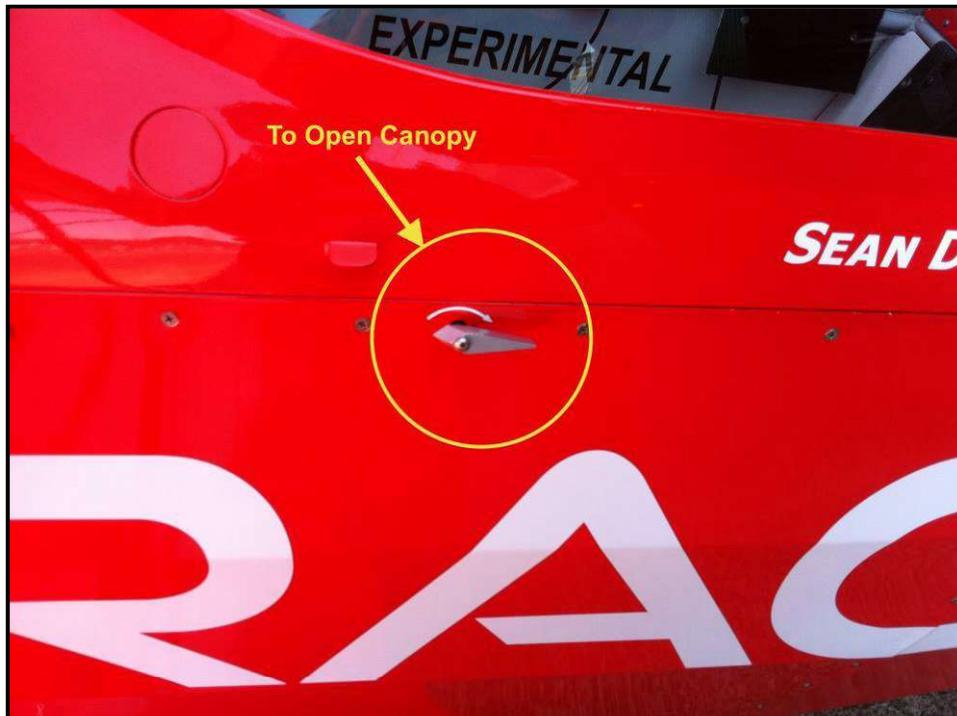
Figure 1 - Canopy Release Lever
