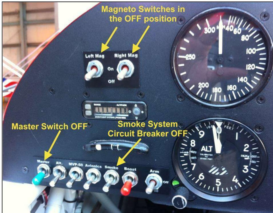
Figure 7 - MASTER & SMOKE SYSTEM switches
