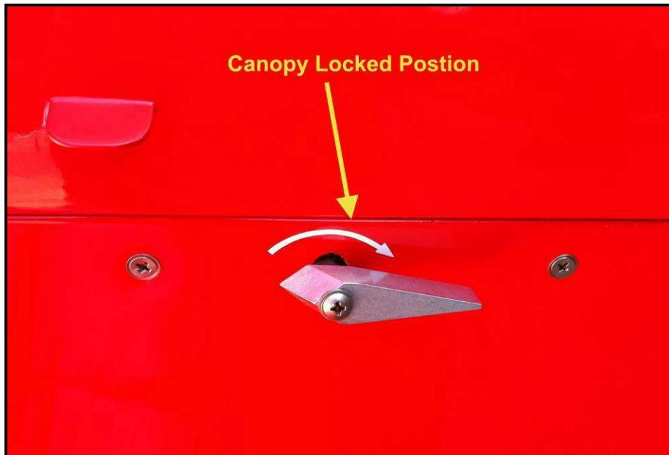
Figure 2 - Canopy **LOCKED** Position
