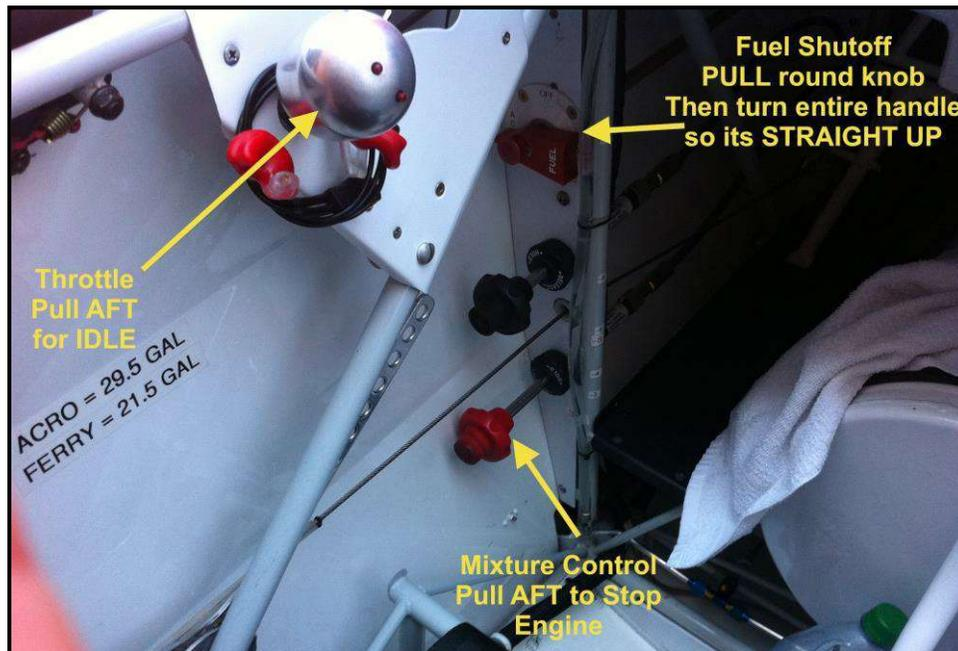
Figure 4 - MIXTURE & THROTTLE knobs
