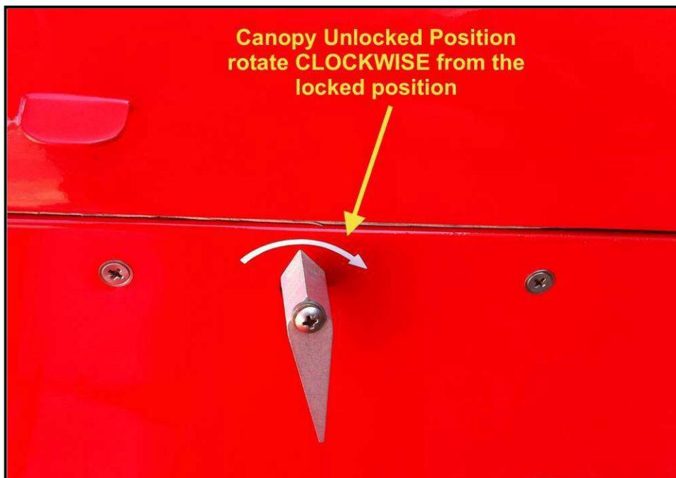
Figure 3 – Canopy **UNLOCKED** Position
