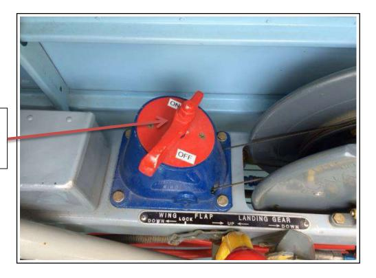
Fuel Selector Valve – Turn Clockwise Down is OFF
