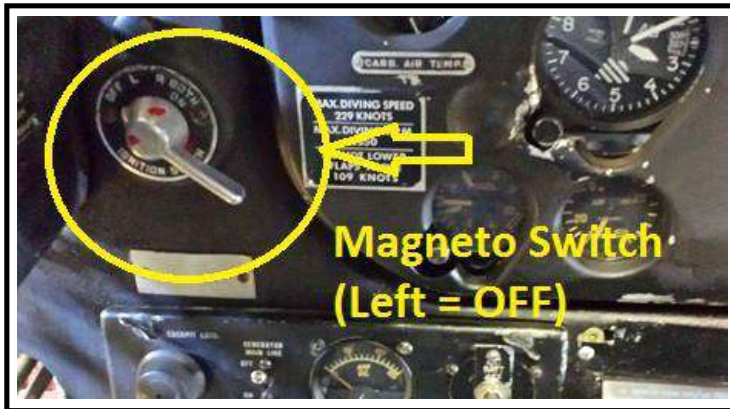
Magneto Switch – Front AND Rear Cockpit, Left Side (switches are interlocked)
