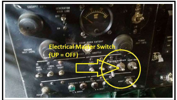
Master (Battery) Switch Front Cockpit, Port Side, Second from Right Up is OFF.
